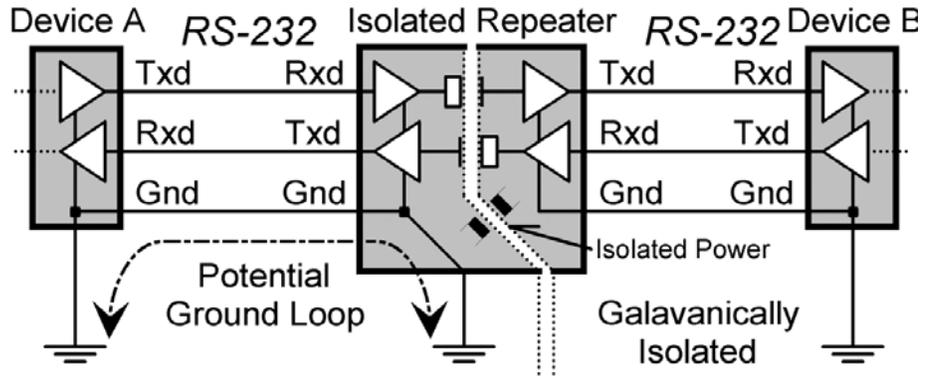
isolated, grounding problems can only be prevented by locating both in the same area and insuring both share a common ground path (one of the assumptions in the EIA/RS-232 standard). 2-port isolation does present another problem; if the isolated repeater shares a DC power supply with other devices, then surges in the common power supply will effect device A through the isolated repeater.
